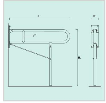
**DESCRIPTION** Folding support bar with vertical rotation, in AISI 304 stainless steel, white finish.
